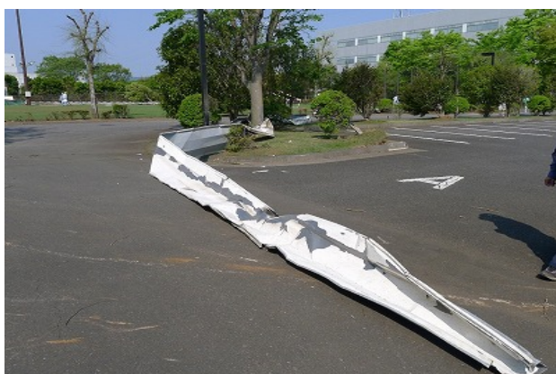
Photo 42 Damage of roofing materials Photo 43 Scattered roofing materials
